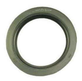
Tides Marine Nitrile Lip Seals are specifically designed for each type of sealing application, whether propeller shaft or rudder stock. They are the only seals which are covered by the Tides Warranty. The outer shell is made of an Aramid fiber composite which is integrally molded to a rubber hinge and a nitrile lip edge. A 316-stainless steel garter spring is incorporated to distribute loads uniformly over the propeller shaft or rudder stock.
